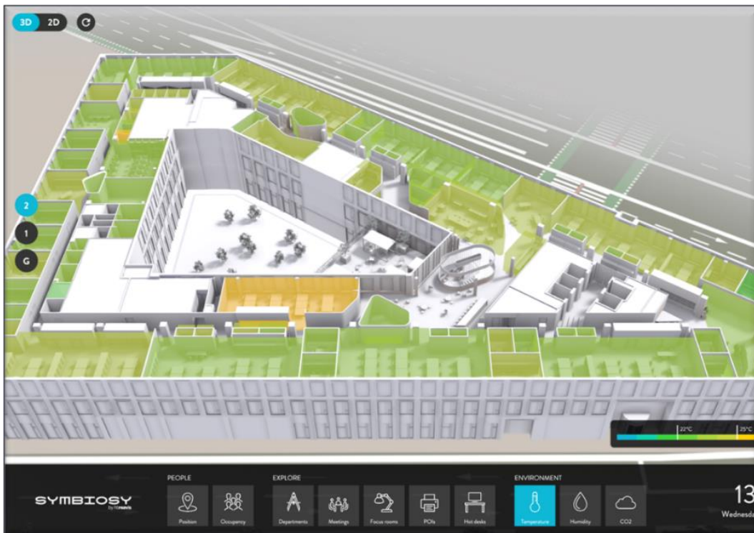
Figure 3: Who is getting frozen out of your office? Temperature in different zones / Image Credit: Symbiosy 3D model screenshot
